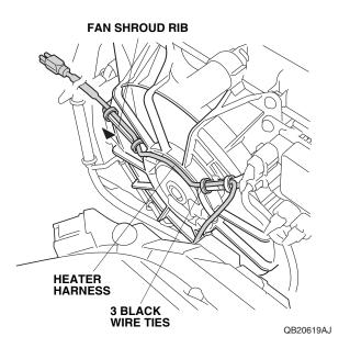
23. Route the heater harness through the front bulkhead, and secure the heater harness to the vehicle harness with one black wire tie.
