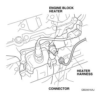
Route the heater harness in the direction shown, and align point A on the heater harness with the vehicle clip. Secure the heater harness to the vehicle harness with one wire tie.
