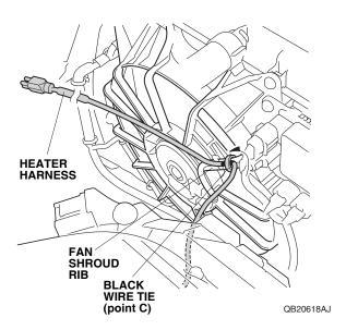
22. Route the heater harness across the fan shroud, and secure the heater harness to the fan shroud ribs with three black wire ties.
