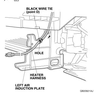
27. Bundle up the heater harness and secure it to the vehicle harness with one black wire tie.
