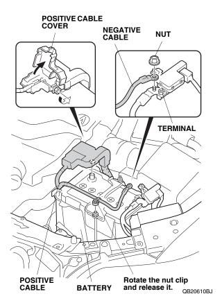
10. Disconnect the negative cable from the terminal (one nut).
