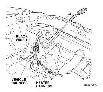
24. Secure the heater harness to the vehicle harness with two black wire ties.
