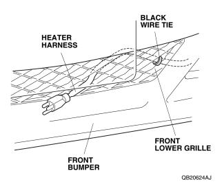
31. Attach the protective cap to the front lower grille, and plug the heater harness connector into the protective cap.
