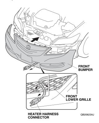
30. Secure the heater harness to the front lower grille with one black wire tie.
