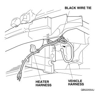
28. Secure the heater harness to the left air induction plate holes with two black wire ties.
